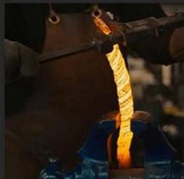
Such repeated folding and forging , greatly improved the toughness of the steel.
