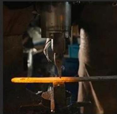
After being smelted into thin sheets, they are folded, twisted and pressed, and then forged again.
