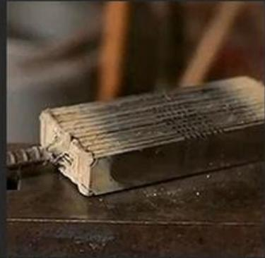
The original steel is pressed and stacked one by one, welded into a whole piece, and then forged at high temperature.
