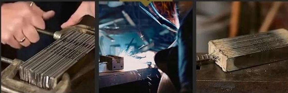
The original steel is pressed and stacked one by one, welded into a whole piece, and then forged at high temperature.
