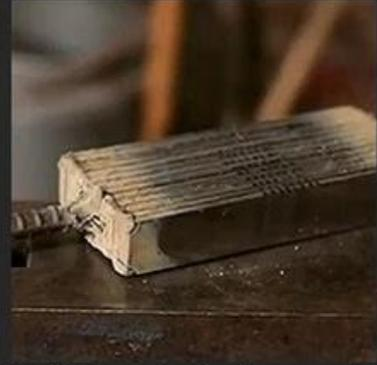
The original steel is pressed and stacked one by one, welded into a whole piece, and then forged at high temperature.
