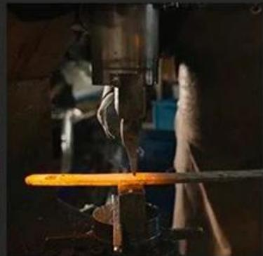
After being smelted into thin sheets, they are folded, twisted and pressed, and then forged again.
