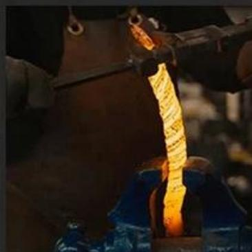
Such repeated folding and forging , greatly improved the toughness of the steel.
