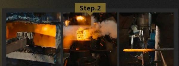
After being smelted into thin sheets, they are folded, twisted and pressed, and then forged again.
