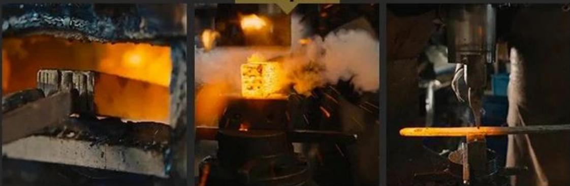
After being smelted into thin sheets, they are folded, twisted and pressed, and then forged again.
