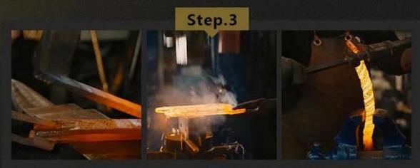
Such repeated folding and forging, greatly improved the toughness of the steel.
