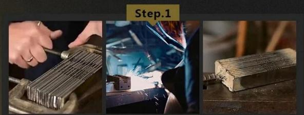
The original steel is pressed and stacked one by one, welded into a whole piece, and then forged at high temperature.
