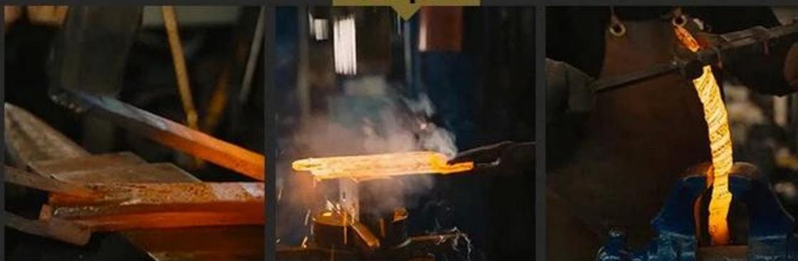
Such repeated folding and forging , greatly improved the toughness of the steel.
