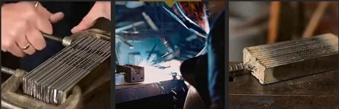
The original steel is pressed and stacked one by one, welded into a whole piece, and then forged at high temperature.
